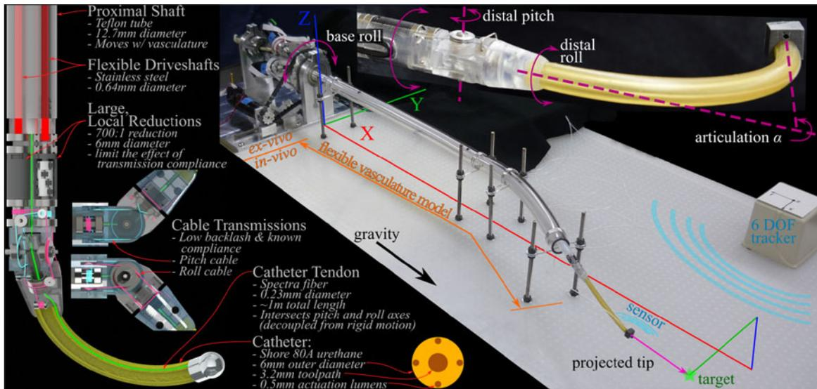
Fig. 2. Five-dimensional prototype interleaved continuum-rigid manipulator. The overall prototype is pictured at center, with the upper-right inset detailing the distal DOF, and the left section views illustrating the mechanical design. See text for further description.
