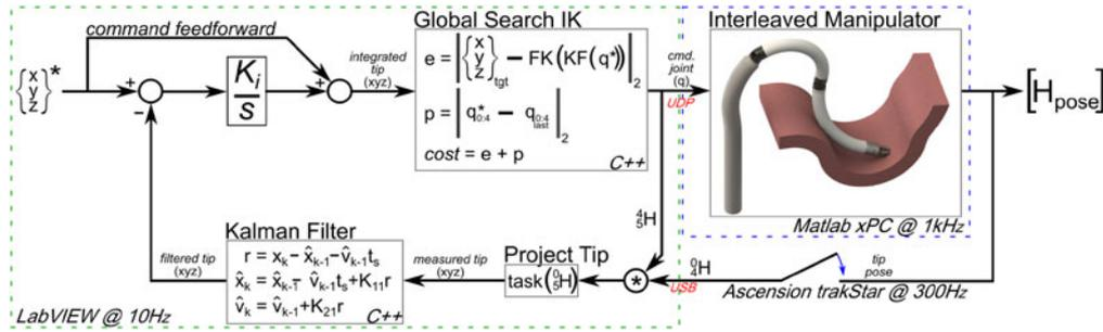
Fig. 3. Multidegree of freedom task space controller. The outer control loop runs at 10 Hz in LabVIEW with the IK and filtering implemented in a C++ library. The servodrives on a MATLAB xPC realtime computer at 1 kHz. The 1-D, 2-state polynomial Kalman filter is used individually on the measured  $xyz$  tip positions and within the IK on the joint angles, each with unique filter gains.
