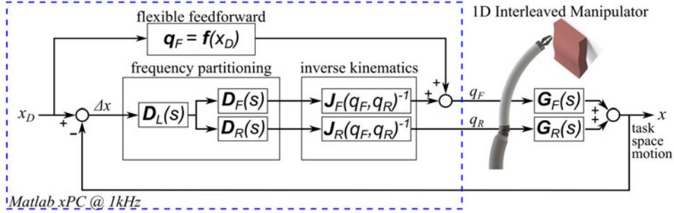
Fig. 7. Overview of a frequency-partitioning single-input multiple-output controller based on [35].
