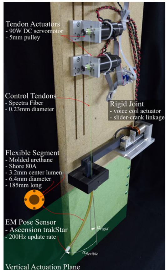
Fig. 6. Single-DOF performance testbed. The 185-mm-long catheter segment is actuated in a vertical plane by two dc motors. The rigid joint moves in the same vertical plane via a slider-crank mechanism actuated by a voice coil. Manipulator articulation is measured by the same electromagnetic pose sensor as before.
