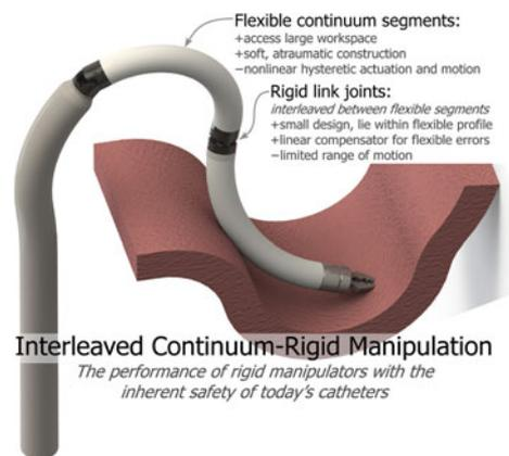
Fig. 1. Notional interleaved continuum-rigid manipulator addressing tissue.
