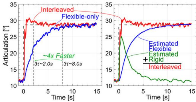
**Fig. 8.** Experimental response of the interleaved testbed to a commanded step of  $17^\circ$  from an initial articulation of  $11.5^\circ$ . Left: Response of interleaved system (red) and response of flexible segment only manipulator (blue); Right: Total response of the interleaved system (red, same as on the left), estimated flexible segment contribution (blue), and estimated rigid-link contribution (green).
